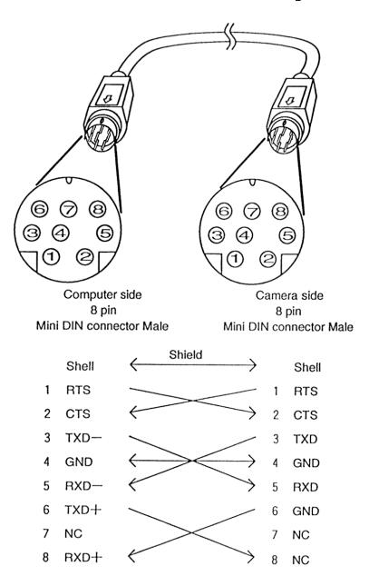
**Note:** RS-232C Specification allows cable length up to 15m, but it should be kept as short as possible.
